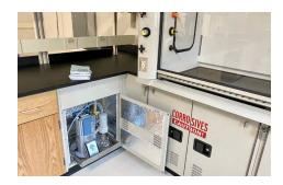
Small, quiet, VACUU•LAN System pumps fit conveniently under a lab bench or fume hood
